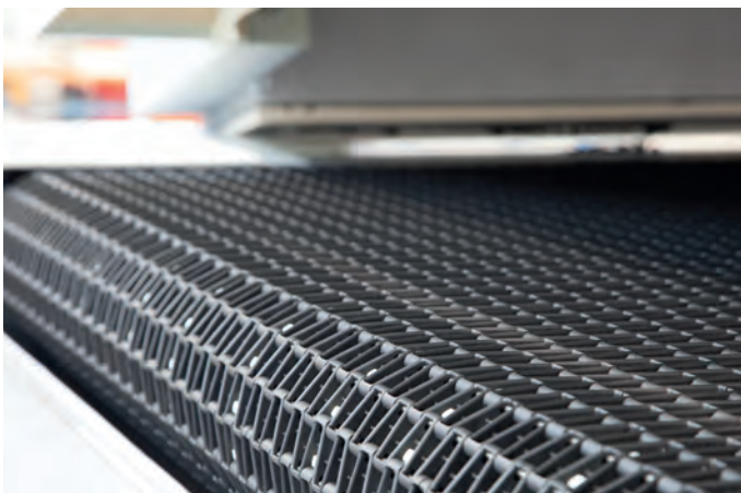
Maintenance-free plastic link belt
