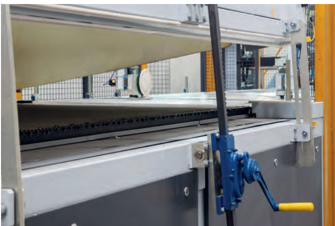
Raising of the tunnel hood
